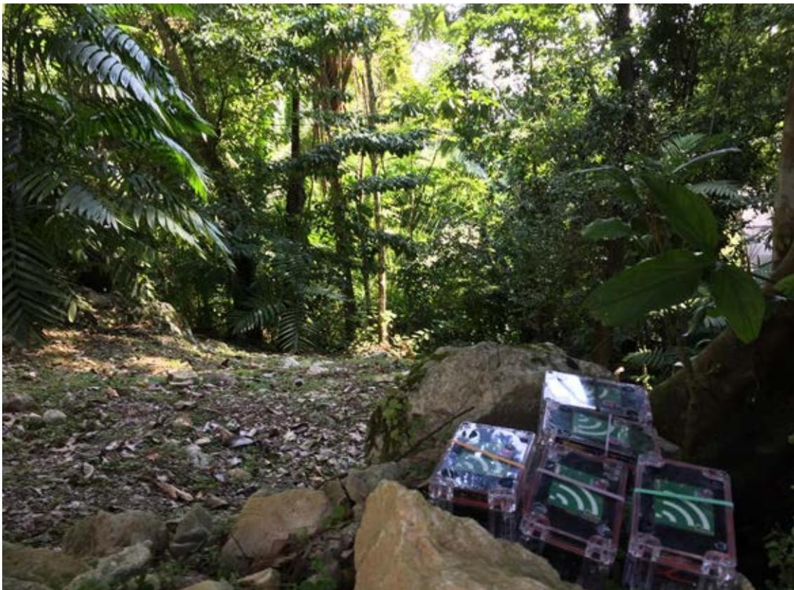
Figure 3. AudioMoth acoustic loggers coupled with GPS modules, here testing satellite signal capture.
