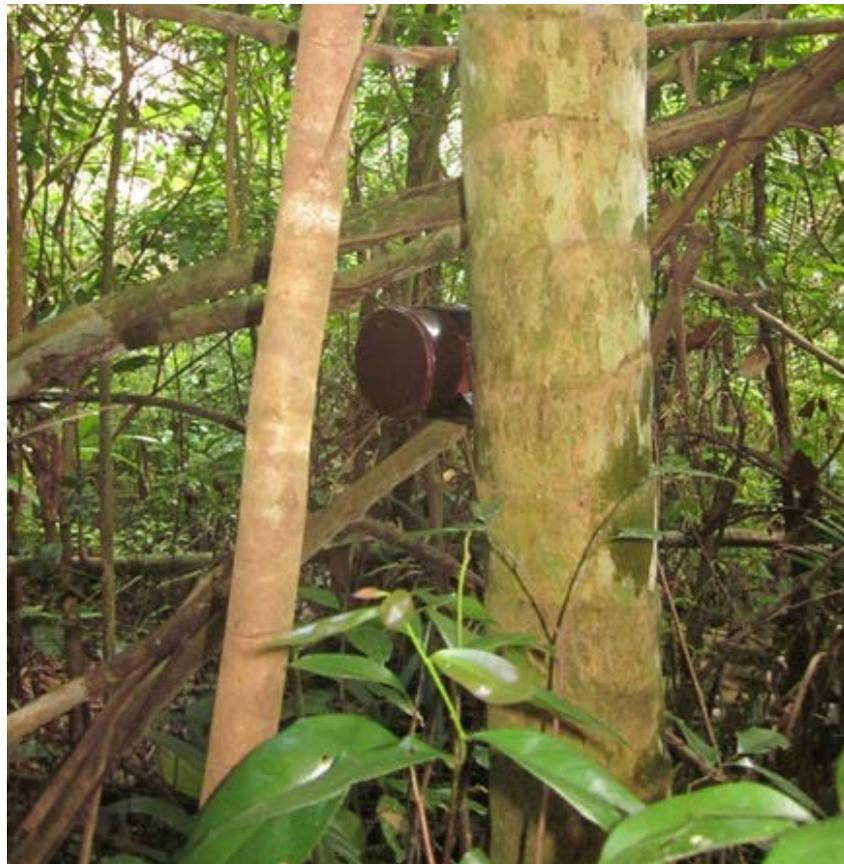
Figure 1. AudioMoth acoustic sensor inside its protective case deployed in Tapir Mountain Nature Reserve.
