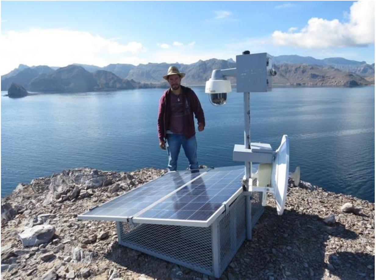
Figure 1. The improved IP camera system, installed at Tijeras island.
