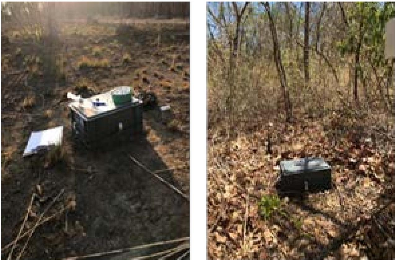
Figure 1. Manual chambers used in the grassland (left) and the forest (right) to measure Greenhouse Gas Emissions in the soil.
