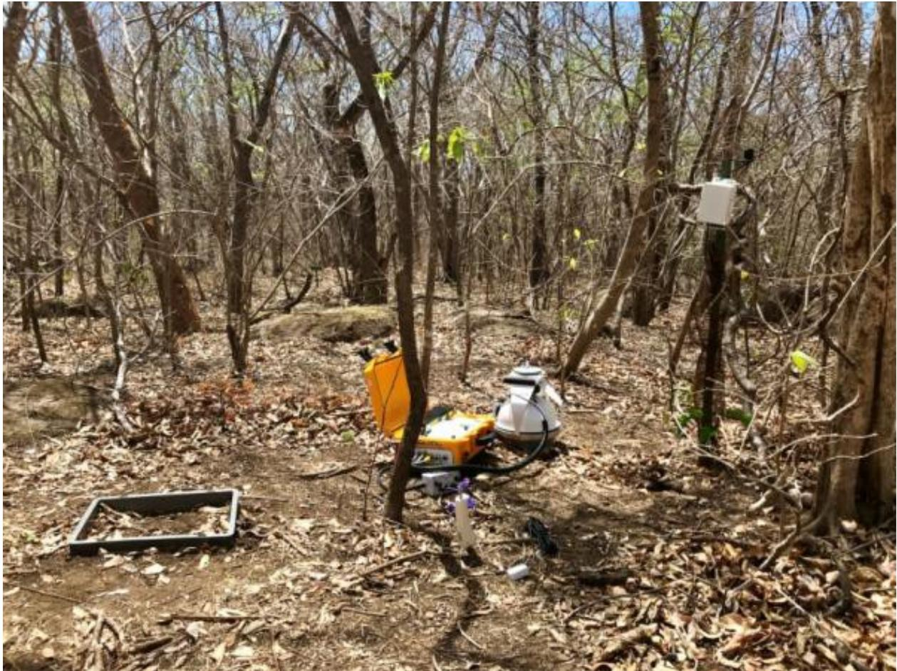
Figure 2. Automatic portable chamber used to measure Greenhouse Gas Emissions in the soil.
